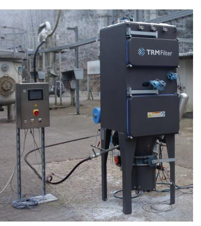
TRM Filter's dedusting unit during live explosion tests at the FSA site in Kappelrodeck.
